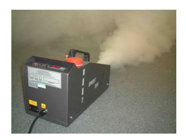
The pump draws Smoke Fluid A (persistent) or Smoke Fluid B (quickly dispersing) from its integral 2 litre reservoir (or an external reservoir if specified), forcing it into the unique precision machined heat exchanger, where it is vaporised. On exiting the heat exchanger, the vapour condenses to form dense, white, non-toxic smoke, with an incredibly consistent, and small particle size of 0.2 - 0.3 micron.
