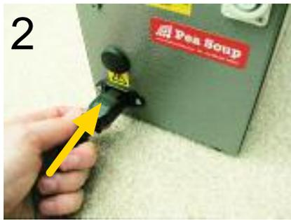
2 Connect to appropriate power supply (230v or 110v - check machine label)
