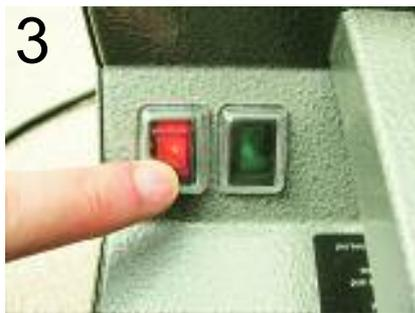
3 Switch the red mains power button to 'on'.
