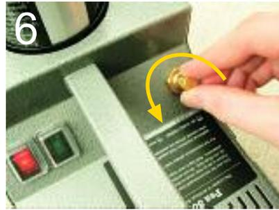
6 For maximum smoke output, adjust flow control to fully anti-clockwise.
